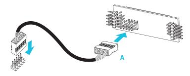
2 Connect the USB 2.0 Cable [B] to the USB1\_3 connector on the DeskMini USB Hub.
